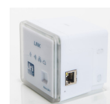
Ethernet socket (absent on WiFi device)
